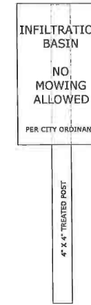
INFILTRATION BASIN SIGNAGE
